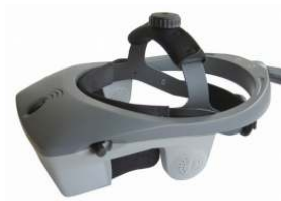
NVIS NVISOR SX [55], binocular 1280x1024, 1kg, 60°. Eye tracker (Arrington Research, [56]) optional (photo courtesy of NVIS)
