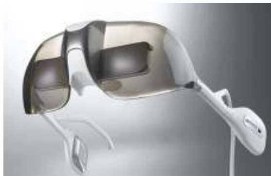
Mirage LightVu [53] OEM optical module for display glasses. The glasses unit weighs 40 grams. The 'nanoprism' assembly (non transparent, see-around) creates a virtual 42" screen from a single display (photo courtesy of Mirage Innovations)
