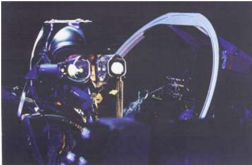
Head Mounted Display System (FOHMD) for out-of-cockpit view of the Tornado Low Level Flight Simulator (photo courtesy of CAE)*
