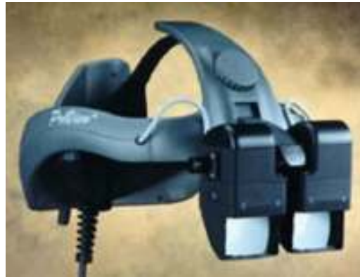
Kaiser Proview XL40 ST: 1024x768 green, 45° diagonal field of view, see-through, 900g (photo courtesy of Rockwell Collins)
