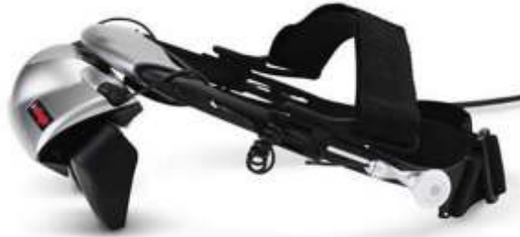
eMagin Z800 3DVisor [60], binocular 600x800 color, OLED on silicon displays, 40° diagonal field of view, equipped with an acceleration based tracking system. (photo courtesy of eMagin Corporation)
