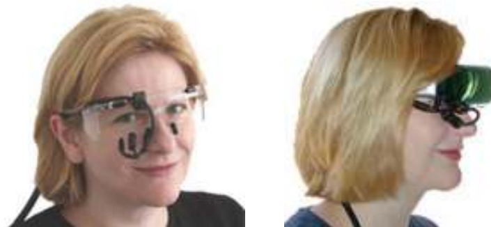
Arrington Research Viewpoint PC-60 eye tracker [56], mounted on glasses and on a HMD
