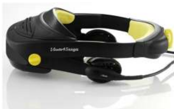
Cybermind Visette 45 XSGA 1280x1024 pixels, 750g, see-through optional (photo courtesy of Cybermind BV)
