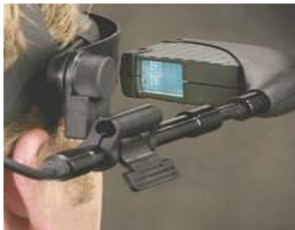
Liteye LE-500 [54]; monocular, 800x600 pixel OLED display, see-through optional, 28° field of view, 120 grams (photo courtesy of Liteye Systems)
