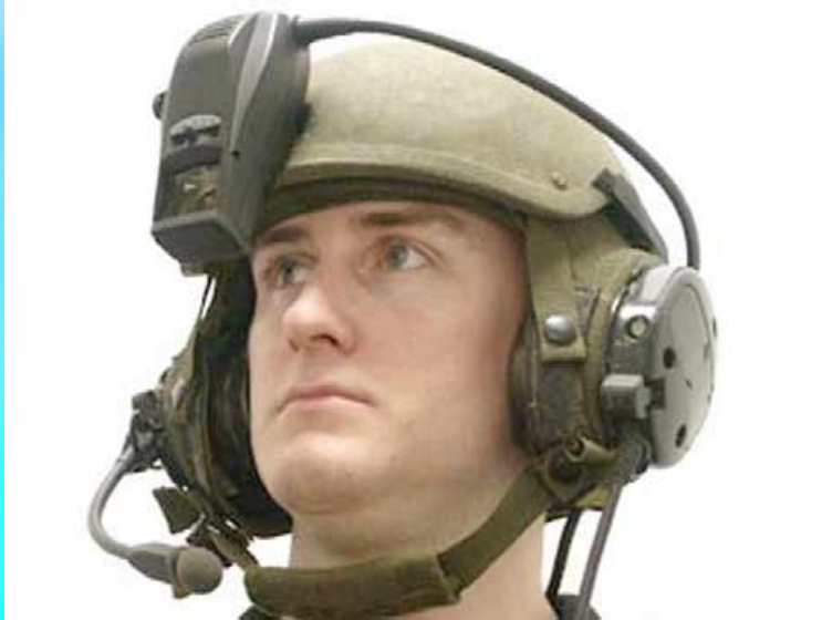
Microvision virtual retina laser displays (monochrome, VGA resolution)
